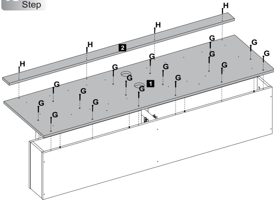
**H** Parafuso Ø3,5x25mm CP **04** **G** Parafuso Ø3,5x40mm CP **16**
