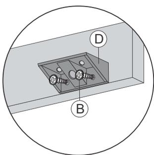
ALINHE O CONECTOR ( D ) NA MOLDURA ( 07 ) E PARAFUSE COM PARAFUSO ( B ).
